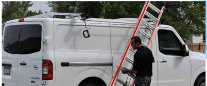
Lower ladder to the ground, resting the top of the ladder on the front bracket.
