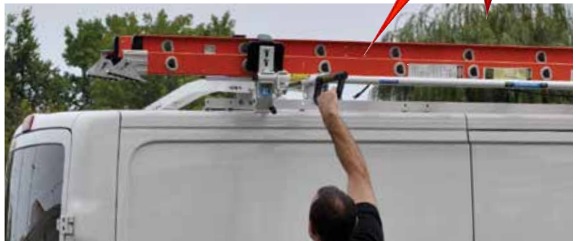
Pull to release the handle, swing out and down to lower ladder.
